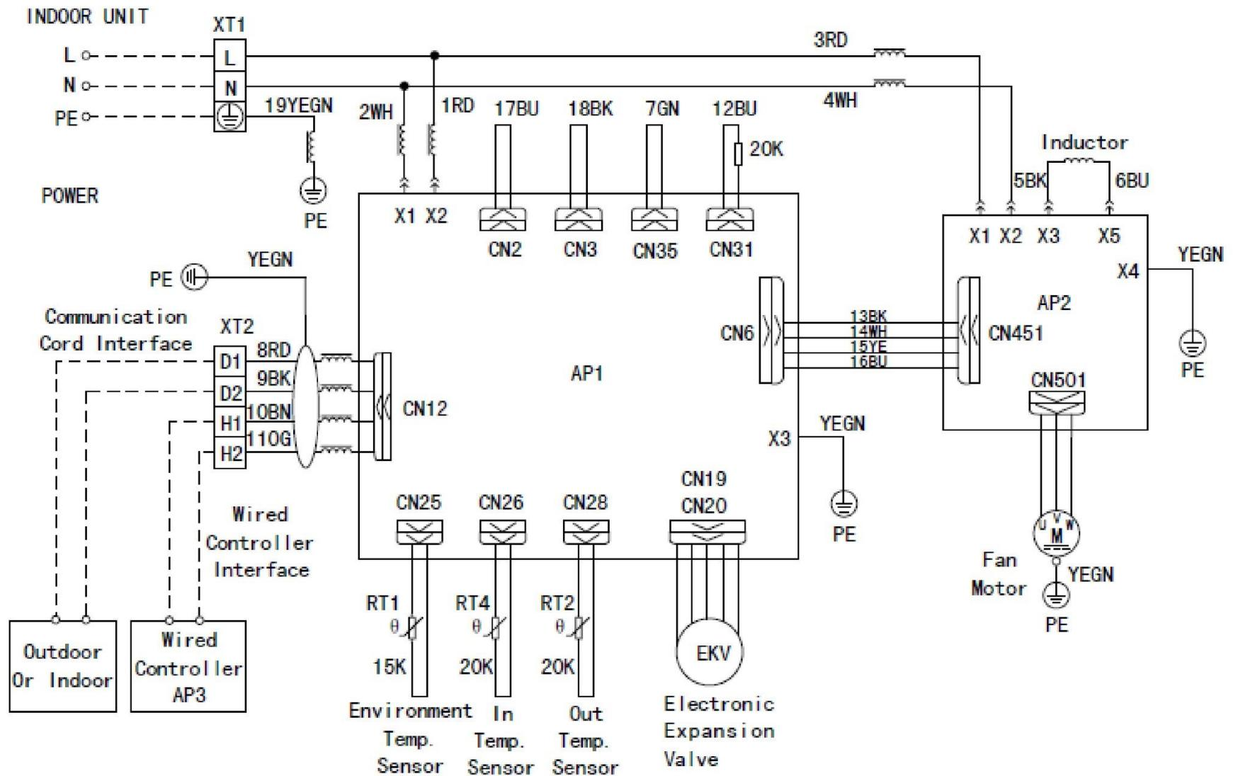
Note: 5-core Electronic expansion valve connect to CN20.
